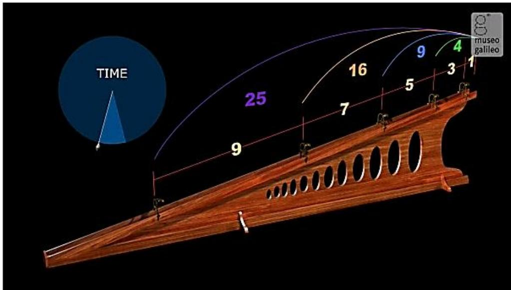
This experimental apparatus provided a demonstration of the Galilean law of the natural fall of bodies, which stated that the spaces traversed from an initial position of rest are proportional to the squares of the times of fall.
